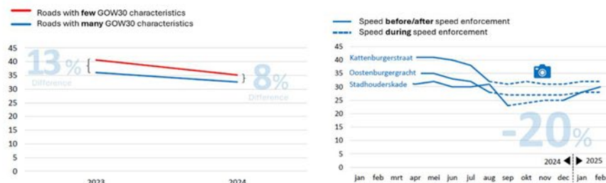
Figure 12: difference in driving speeds in relation to road characteristics (left) and effect of speed enforcement (right)
